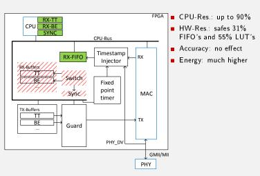
HW/SW Co-Design for TDMA Ethernet controllers
